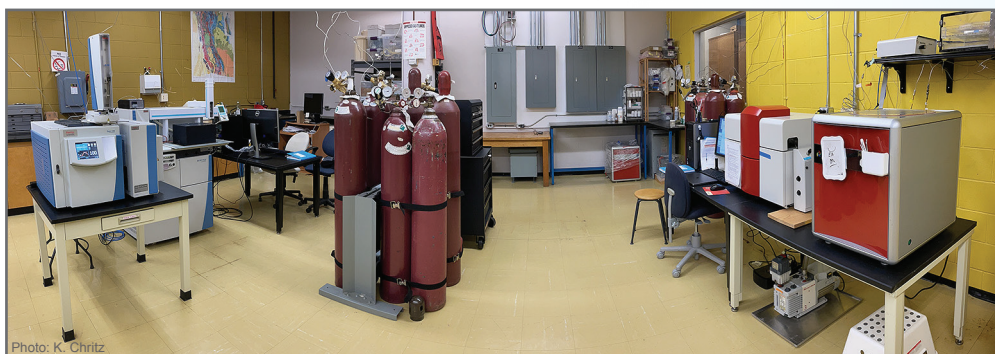
Thermo Fisher Scientific Delta V Plus IRMS (left) with GCC and GasBench; Isoprime 100 IRMS (right) with EA
